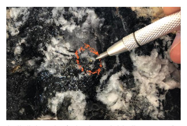
The visible gold in the picture above is from the A pit (westernmost) and is hosted by a pegmatitic quartz-albite-biotite vein. The outcrop that was blasted at this location returned several channel assays in the 1-3g/t Au range from a combination of blue quartz veins, and pegmatitic veins with arsenopyrite disseminations.
